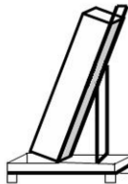
Fig (2): Schematic of steel stainless mould and fixture
